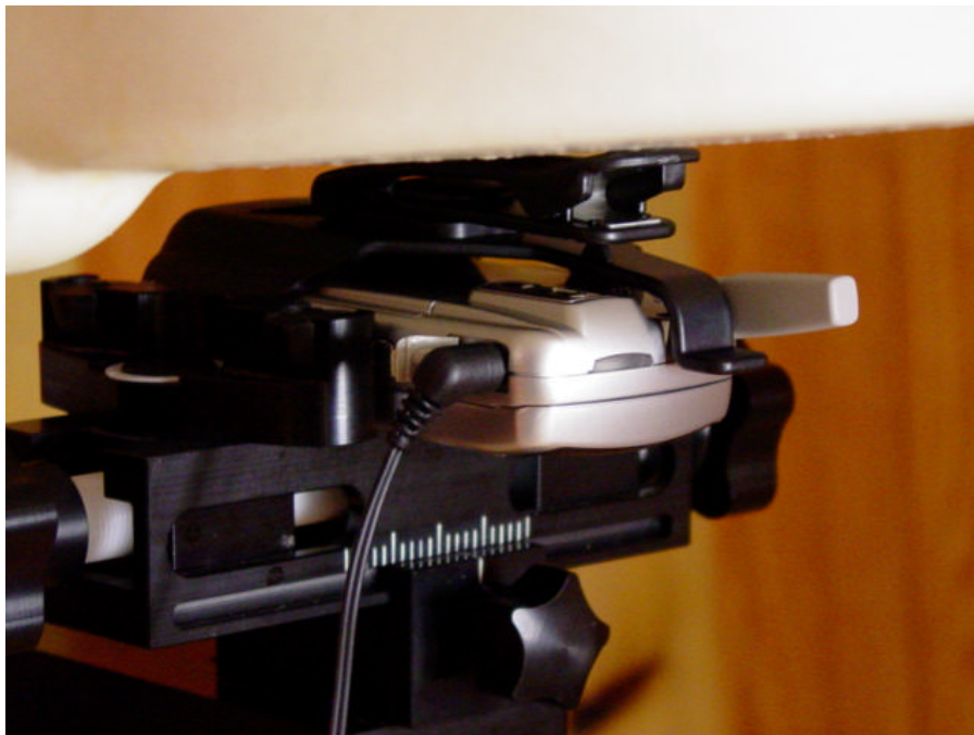
Figure 12.5 body SAR setup (with holster)
