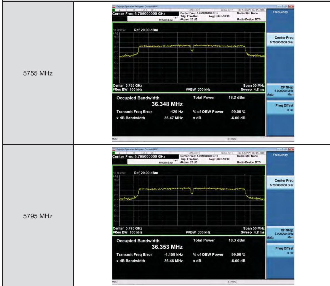
**Maximum Power Spectral Density Measurement**
