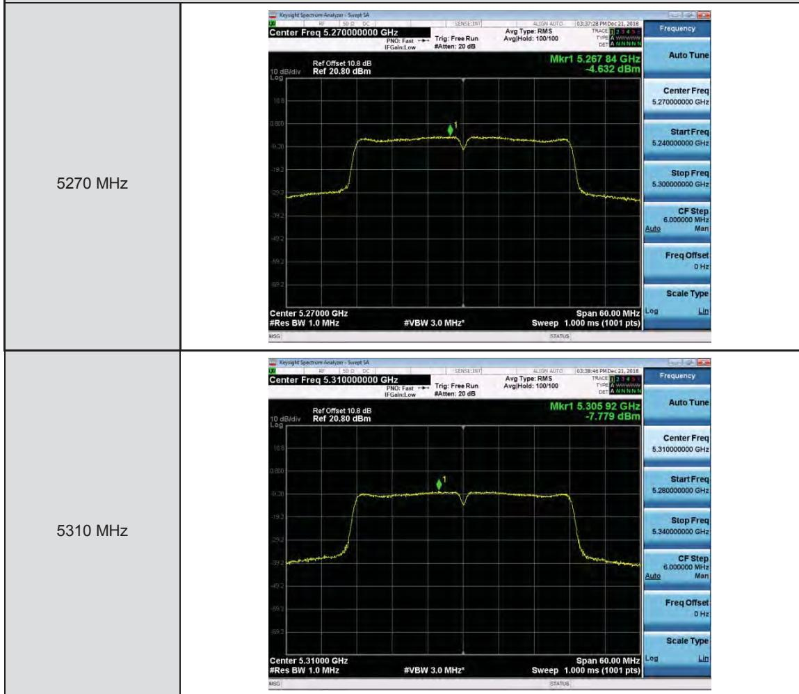
Mode 4: IEEE 802.11n 5 GHz 40 MHz Continuous TX mode\_ ANT-0
