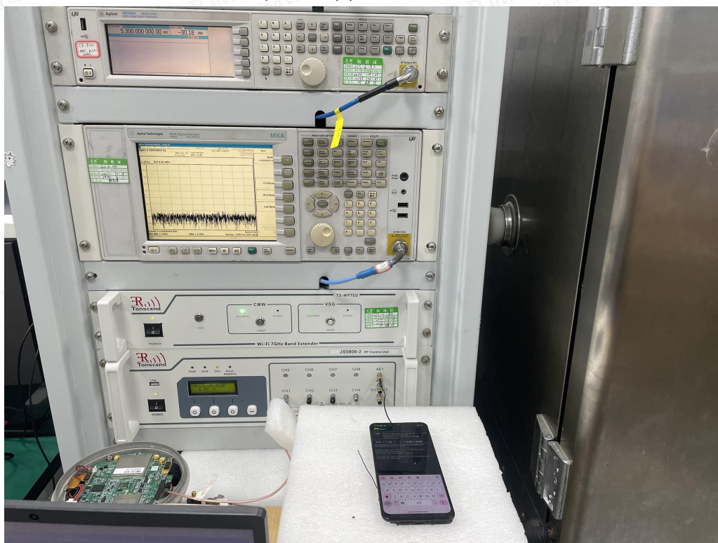
Test Setup Photo(s) of DFS Measurement
