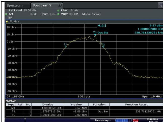
GSM 1900 VOICE Middle Channel
