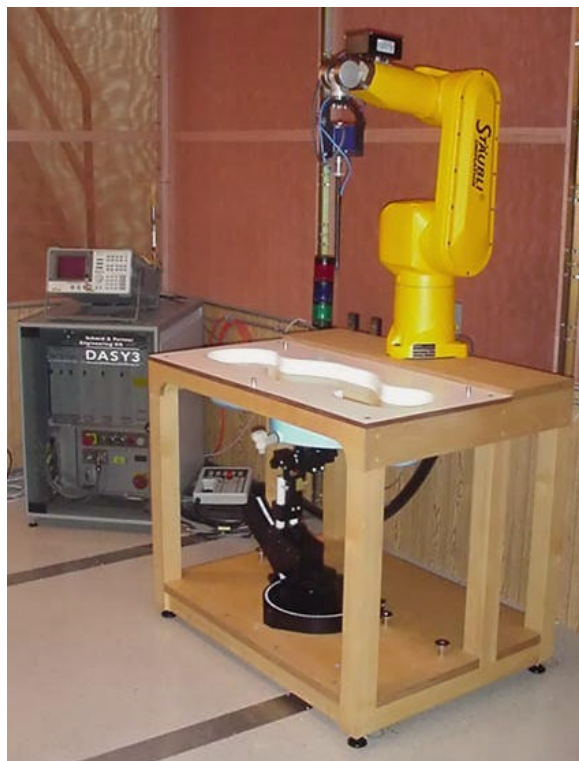
DASY3 SAR Measurement System
