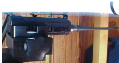
Body-worn SAR Test Setup with 1.0cm Belt-Clip
