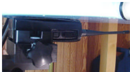
Body-worn SAR Test Setup with 0.9cm Belt-Holster
