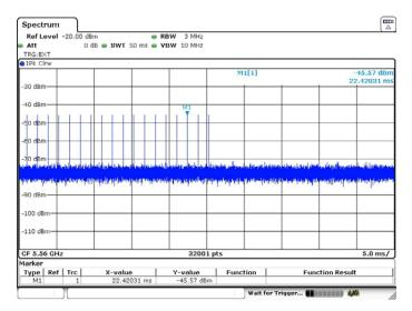
Peak of -45.57dBm, with losses at combiners factoring antenna gain to be 15.81dB, therefore level going into antenna port is -61.38dBm which exceeds threshold level of -64dBm for successful detection.
