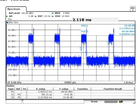
The resulting plot data was extracted and post processed, giving a duty cycle of 20.13%.
