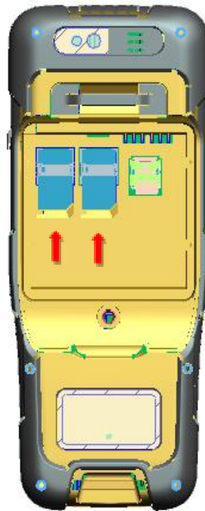
Figure 2.16 Put the SIM card in the holder
