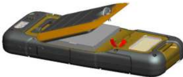
Figure 2.15 Take off the back cover
