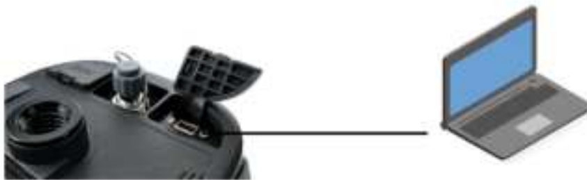
Figure 2.12 Connect Oscar to a computer
