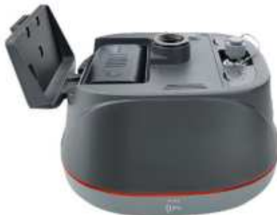
Figure 2.2 Put one battery in Oscar
