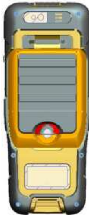
Figure 2.18 Insert the back cover
