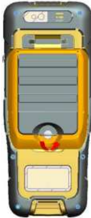
Figure 2.14 Remove the back cover
