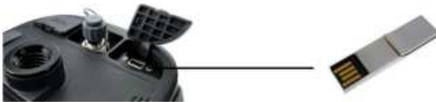
Figure 2.13 Connect Oscar to a USB memory stick
