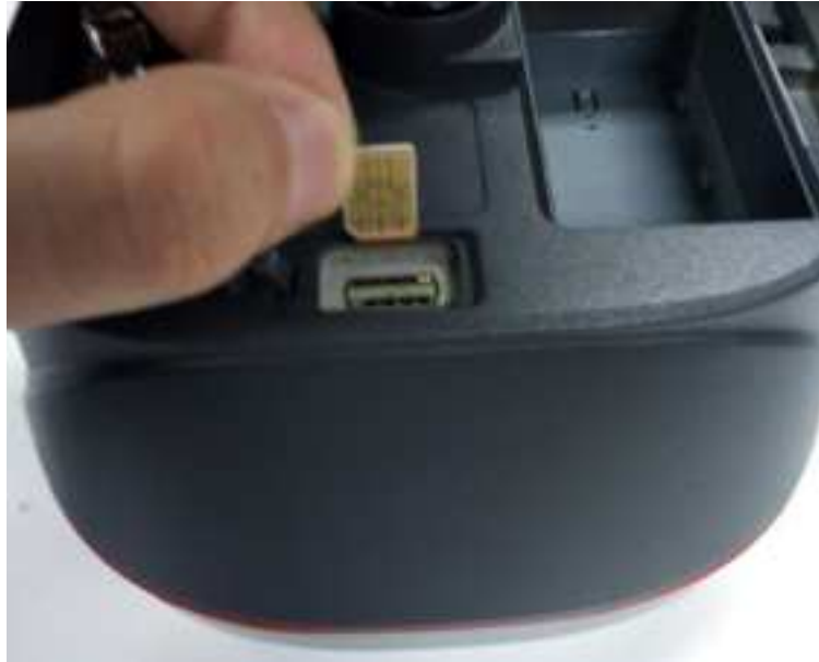
Figure 2.3 Insert the SIM card
