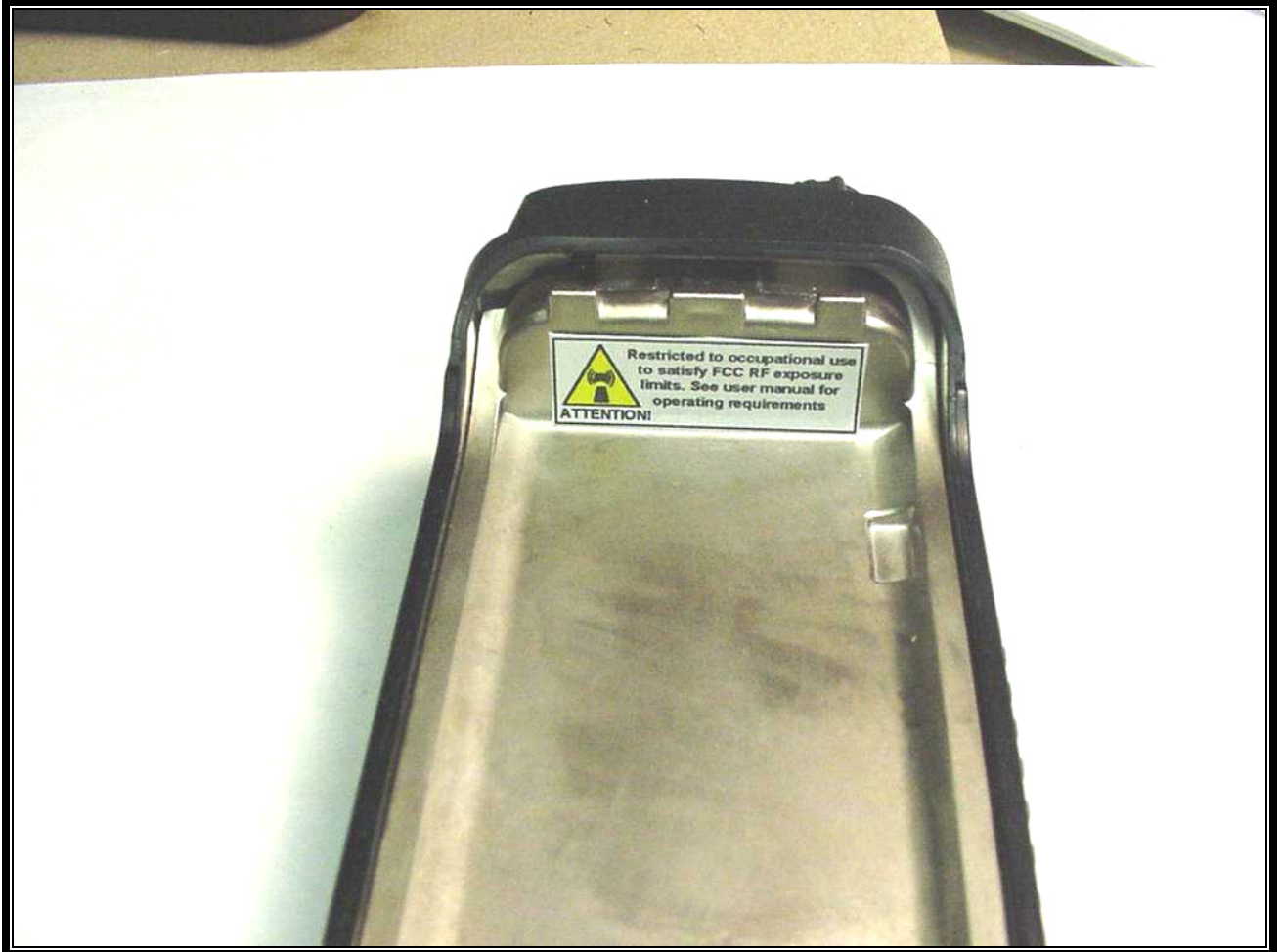
PHOTOGRAPH 2: RF LABEL AND LOCATION
