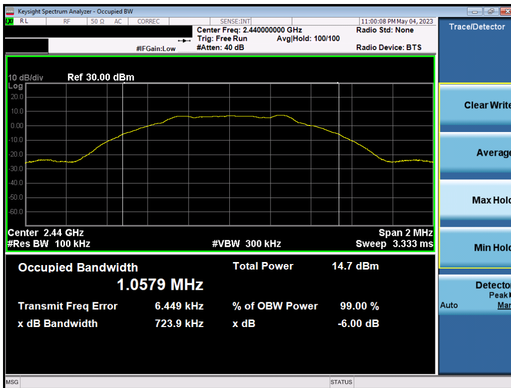
Plot 7-14. 6dB BW & 99% OBW Plot NB UNII_L (Bluetooth (LE), 1Mbps, iPA – Ch. 19)
