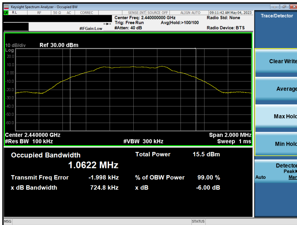
Plot 7-2. 6dB BW & 99% OBW Plot Ant1 (Bluetooth (LE), 1Mbps, ePA – Ch. 19)
