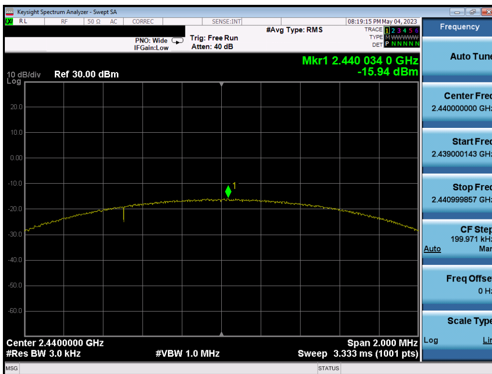
Plot 7-69. Power Spectral Density Plot Ant1 (Bluetooth (LE), 2Mbps, iPA – Ch. 19)
