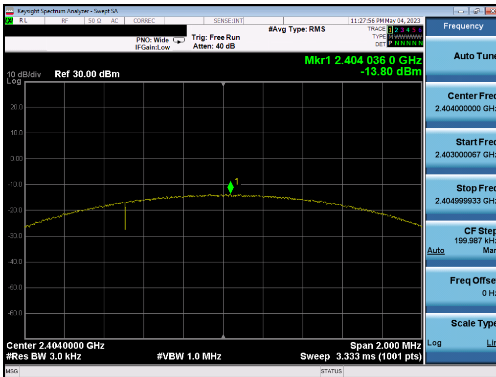
Plot 7-46. Power Spectral Density Plot NB UNII_L (Bluetooth (LE), 2Mbps, iPA – Ch. 1)
