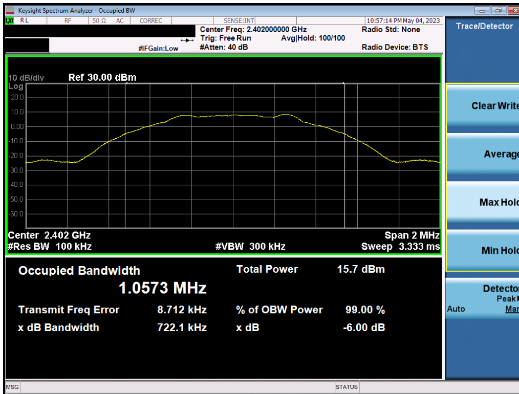
Plot 7-13. 6dB BW & 99% OBW Plot NB UNII_L (Bluetooth (LE), 1Mbps, iPA – Ch. 0)
