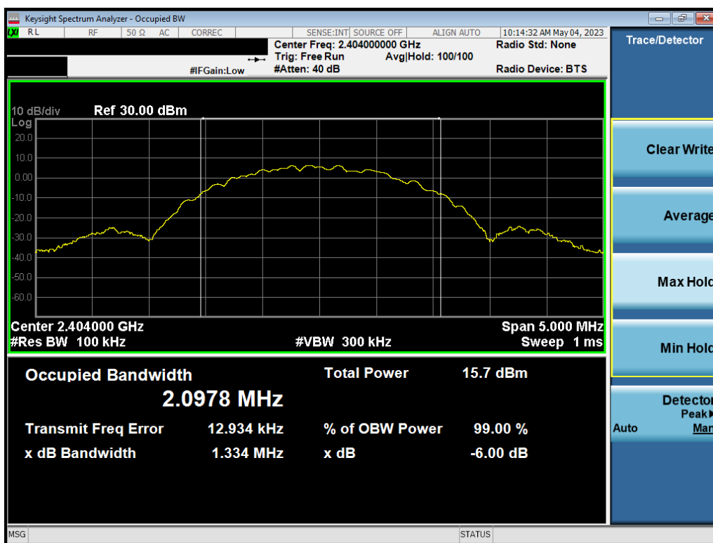
Plot 7-4. 6dB BW & 99% OBW Plot Ant1 (Bluetooth (LE), 2Mbps, ePA – Ch. 1)
