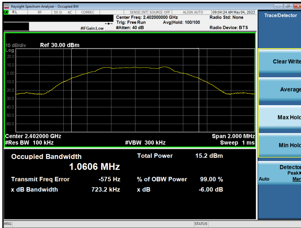
Plot 7-1. 6dB BW & 99% OBW Plot Ant1 (Bluetooth (LE), 1Mbps, ePA – Ch. 0)
