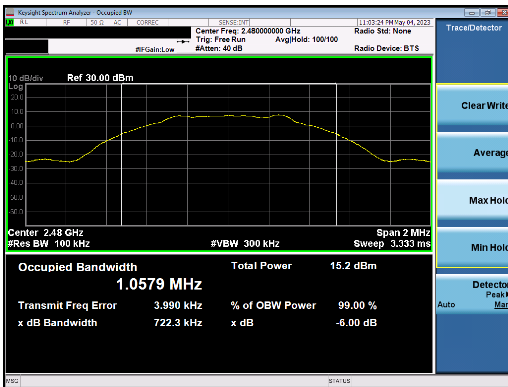
Plot 7-15. 6dB BW & 99% OBW Plot NB UNII_L (Bluetooth (LE), 1Mbps, iPA – Ch. 39)
