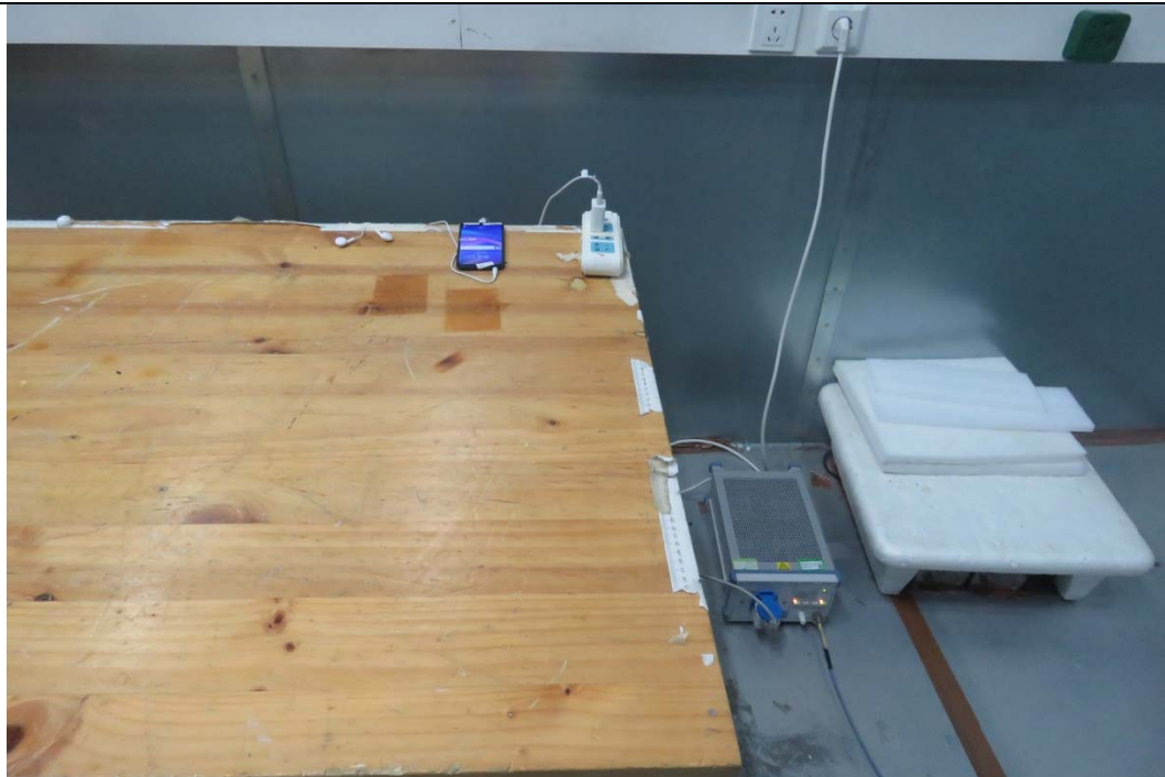
Picture 2 Conducted Emission Test Setup
