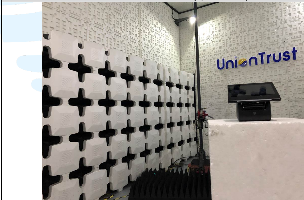
Radiated emission Test Setup (Above 1 GHz)
