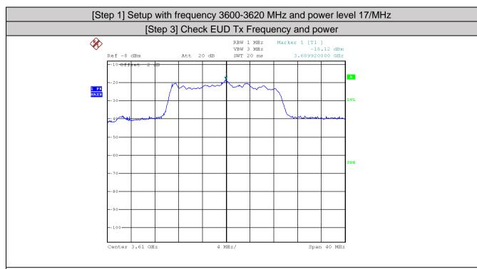
EIRP=Conducted Power + Loss + Directional Antenna=-18.12+5+3+6.02=-4.1dBm/MHz
