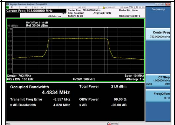
LTE band 14 - Low CH 16QAM-5
