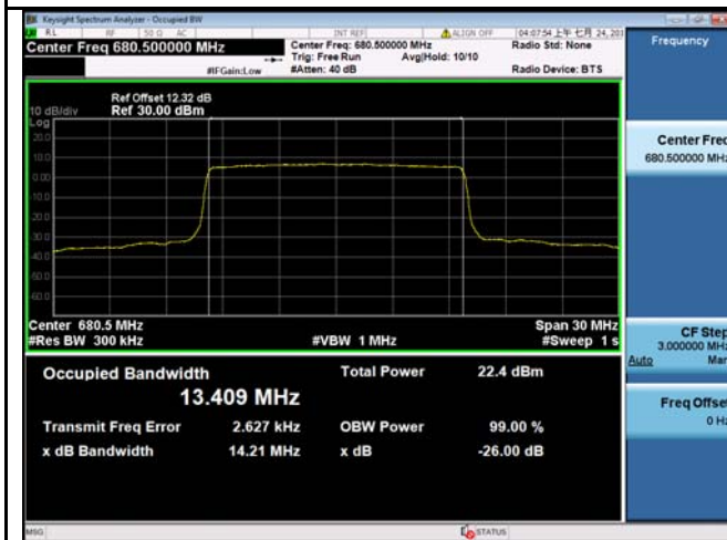
LTE band 71 - Low CH QPSK-15
