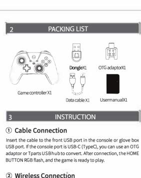
a.) First pairing: Long press the HOME BUTTON 3-5 seconds to start the pair mode, insert the dongle to the front USB port in the console or glove box USB, click the button in the dongle to make the pairing happen. After connection, the HOME BUTTON will be onstill, and the game is ready to play
