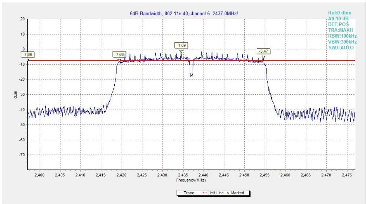
Fig.A.4.11 Occupied 6dB Bandwidth (802.11n-HT40, Ch 6)
