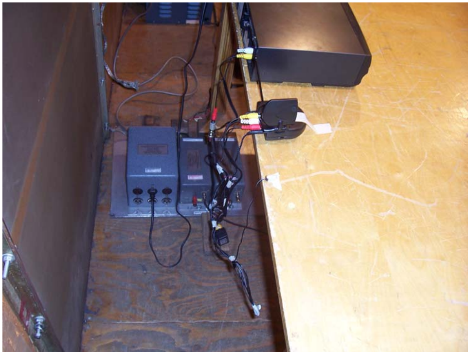
Conducted Emissions, Rear Test Setup
