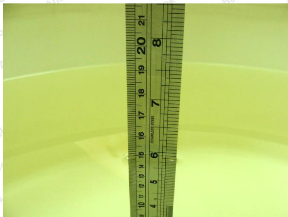
Photo of Liquid Height for Body SAR
