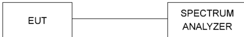
Figure 1 - Bandwidth Measurements Test Setup
