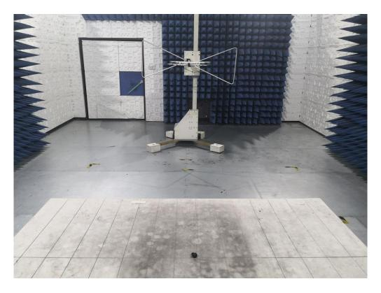
RADIATED EMISSION TEST SETUP ABOVE 1GHZ
