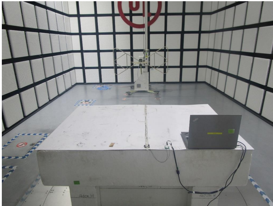
RADIATED RF MEASUREMENT SETUP (Below 30MHz)
