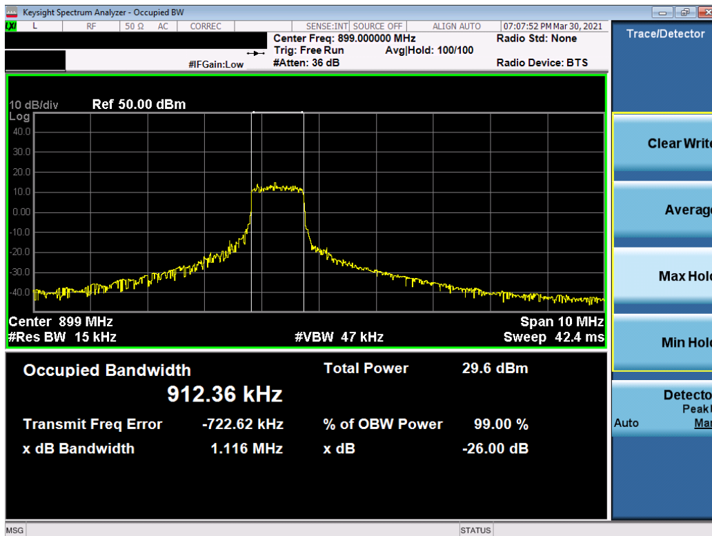
Plot 7-3. Occupied Bandwidth Plot (3MHz, 16-QAM, RB 5, RB Offset 0, NB=0)
