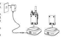
Warning: Never charge while the radio is turned on. When turned on, the charger can't detect the charging voltage properly and LED fails to indicate charge status correctly.
