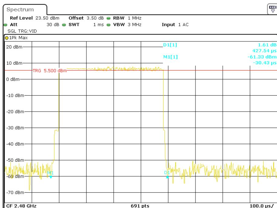
**Pulse time, Low Channel, 2DH3**
