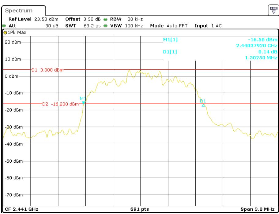
**EDR ( $\pi/4$ -DQPSK): High Channel**
