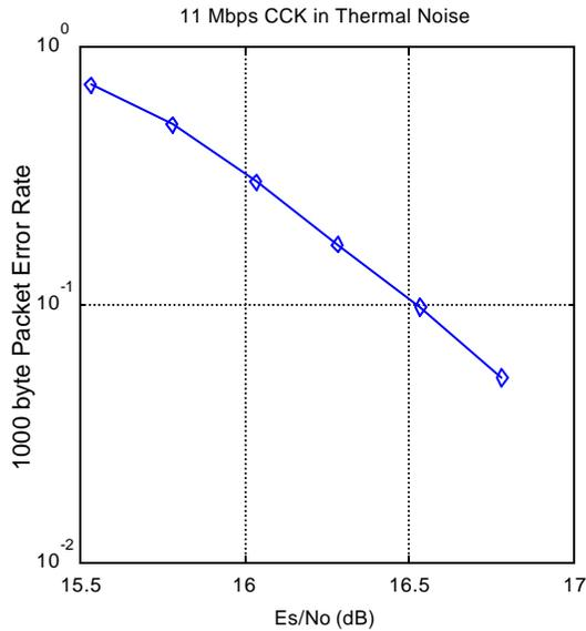
The reference PER is specified as 8% . The corresponding Es/No (signal to noise ratio per symbol) is 16.4 dB. The Es/No required to achieve the desired PER with maximum system implementation losses is 18.4 dB. The minimum processing gain is again, 10 dB, therefore:
