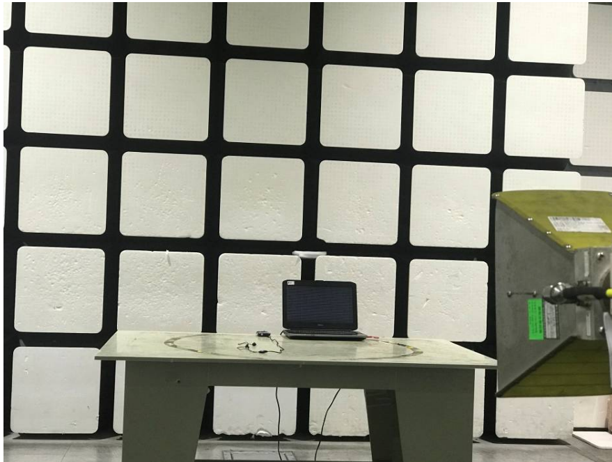
Radiated Emissions - Front View (Above 1 GHz)
