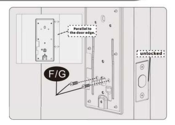
Secure the mounting plate with the supplied screws.
