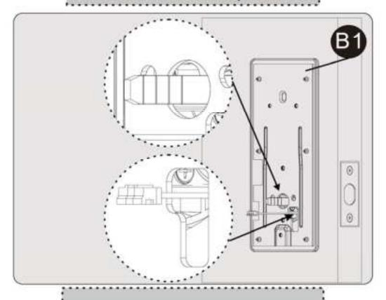
Route the cable through the hole in the mounting plate.
