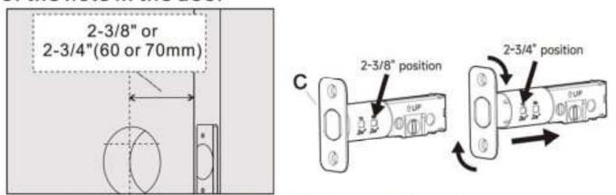
B:Secure the latch (C) and buckle box (C1) to the corresponding holes in the opened door with 2\*tapping screws (E).
