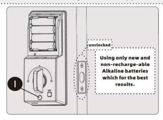
While the door is open and unlocked, load 4 AA batteries into the interior assembly. And then the latch bolt will extend to learn the orientation of the door.
