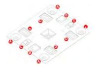
FIGURE 3 AP Securely Attached to T-bar
