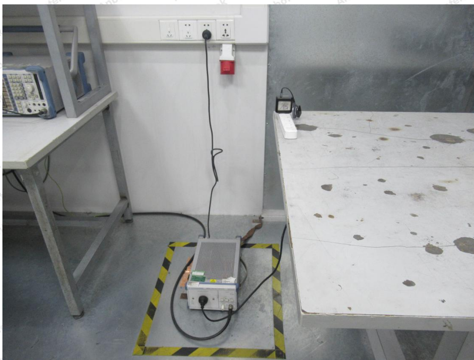
Photo of Conducted Emission Measurement
