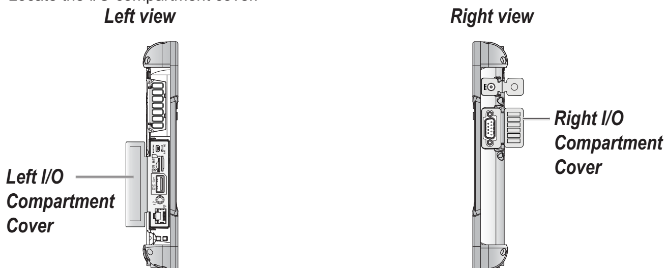
Figure 26. Side View: Locating the I/O Compartment Cover
