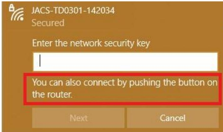
You can press the WPS button on the TD0301 until the Wi-Fi light flashes quickly, to activate the WPS, then you can see the connecting process.
