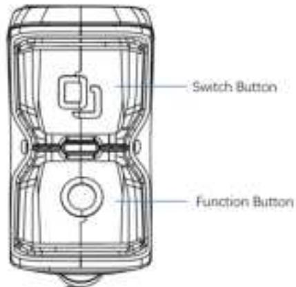
**Switch Button:** Press once to switch the home page and data page. Press and hold to enter/exit Settings.
