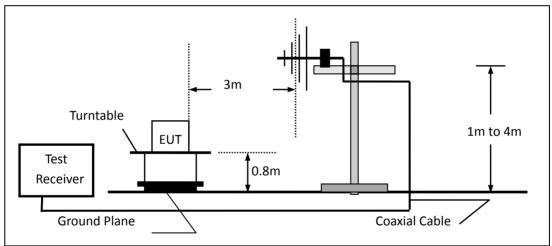
(c) For radiated emissions above 1000MHz
