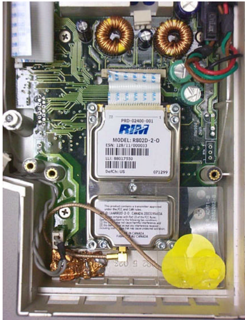
Lipman USA, Ltd. Nurit 3010 with DataTAC modem
