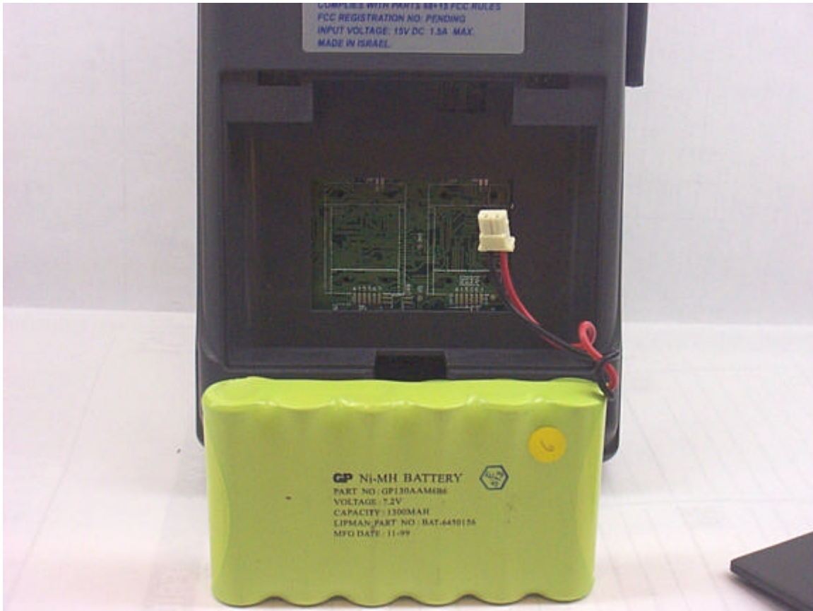
Lipman USA, Ltd. Nurit 3010 Battery compartment open
