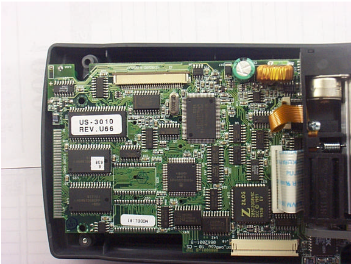
Lipman USA, Ltd. Nurit 3010: Board over modem
