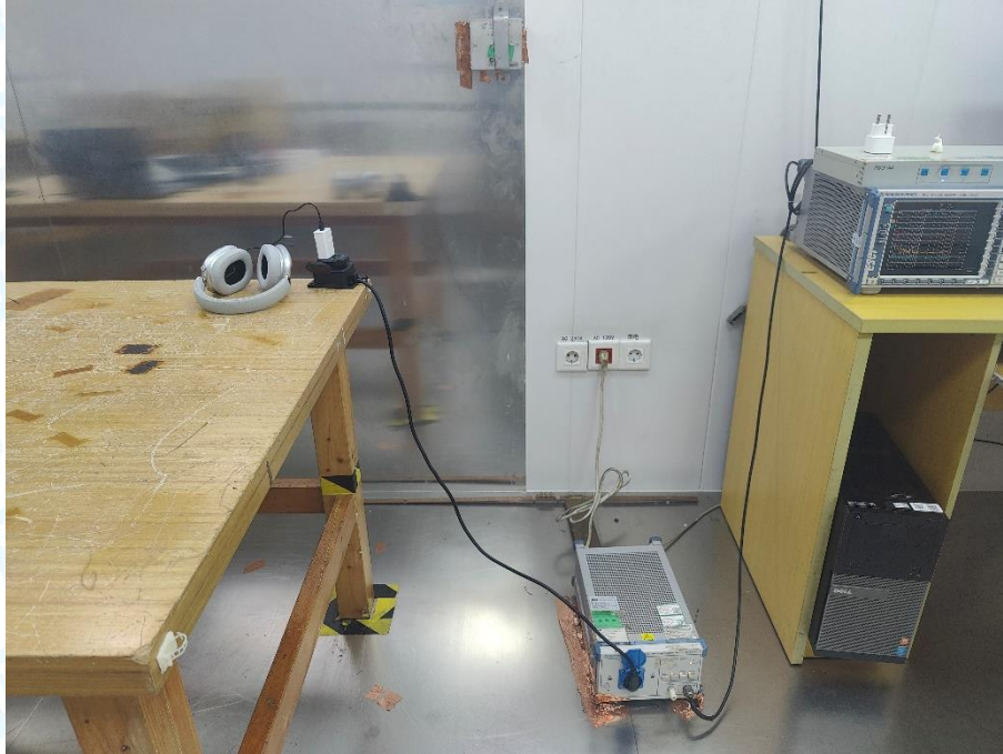
Photo of Setup for Radiated Emission (30MHz~1GHz)
