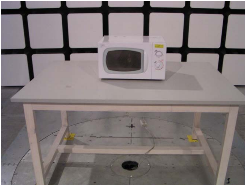
30 MHz to 1000 MHz- Radiated Emission–Rear View
