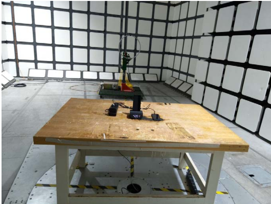
Radiated Emissions View (9 kHz ~ 30 MHz)
