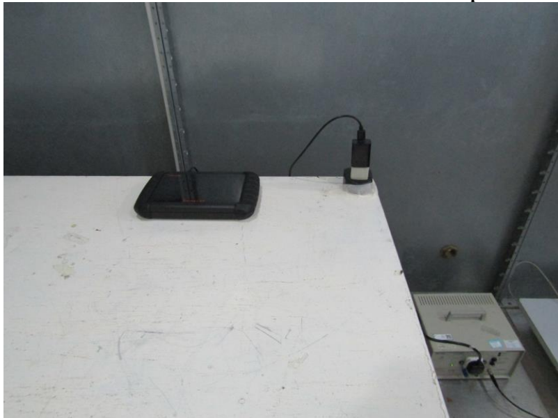
Measurement of Conducted Emission Test Set Up
