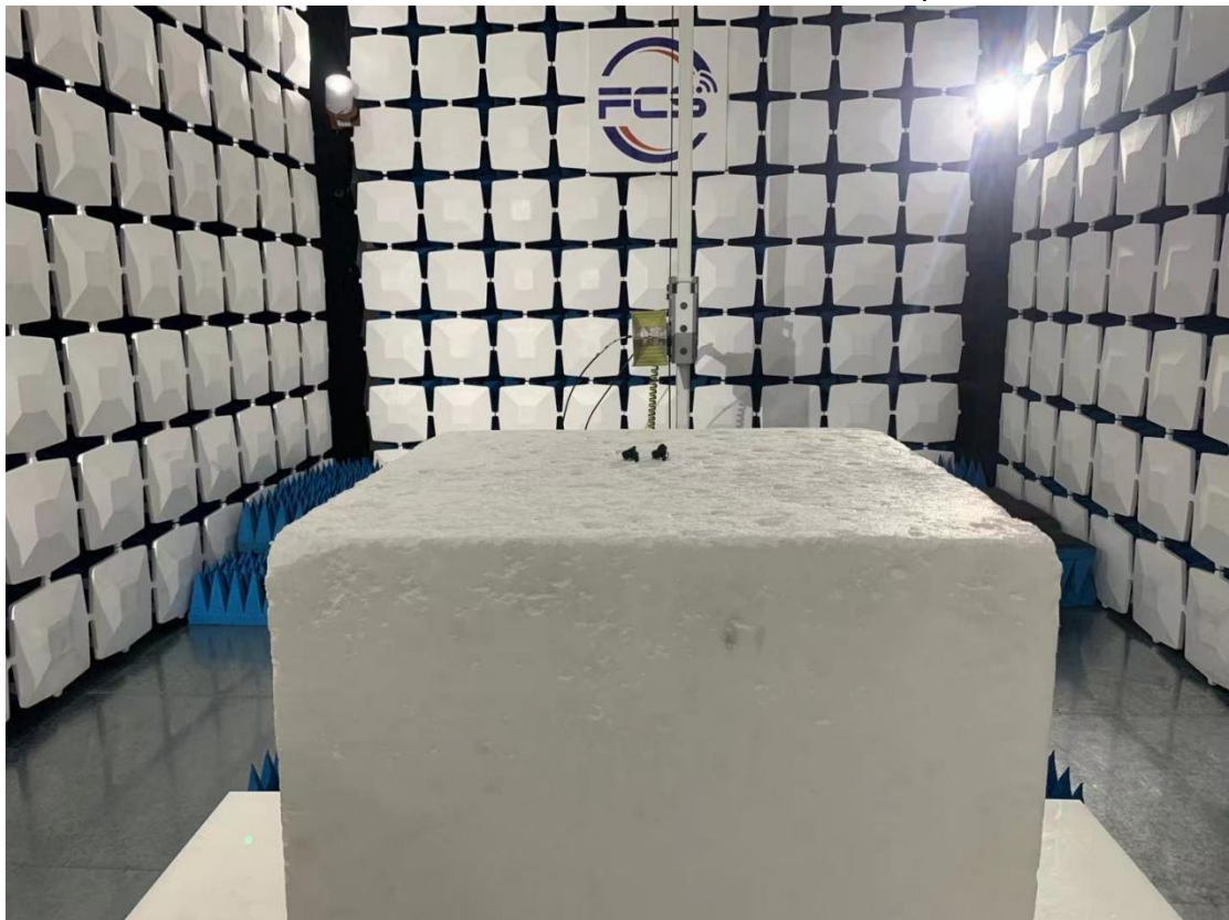
Above 1GHz for radiated emission test setup
