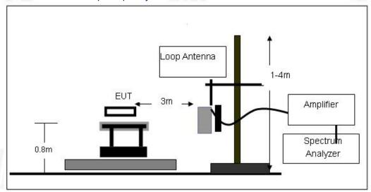
(B) Radiated Emission Test-Up Frequency 30MHz~1GHz
