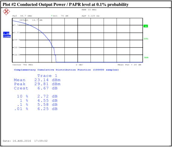
Note: Offset in this measurement should be 12.9 dBm which is reflected in the data table of section 6.4. Output power after accounting for external attenuation is 21.3 dBm.
