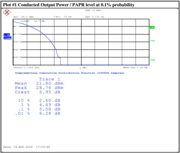
Note: Offset in this measurement should be 14.4 dBm which is reflected in the data table of section 6.4. Output power after accounting for external attenuation is 21.5 dBm.
