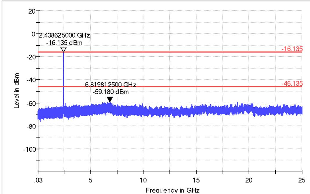
In any 100kHz bandwidth, the Conducted Spurious Emissions from 30 MHz to 25 GHz were greater than 30dB below the peak emission within the band that contains the highest level of the desired power.
