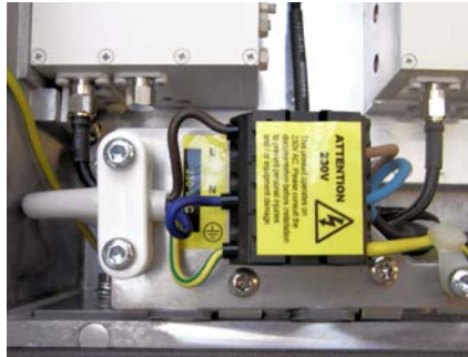
Figure 3-17: 230 VAC Power Connections
