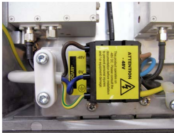
Figure 3-19: -48VDC Power Connections
