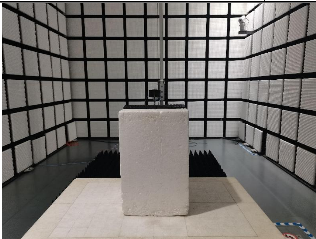
Fig. 3 Radiated emission setup photo(Above 1GHz)
