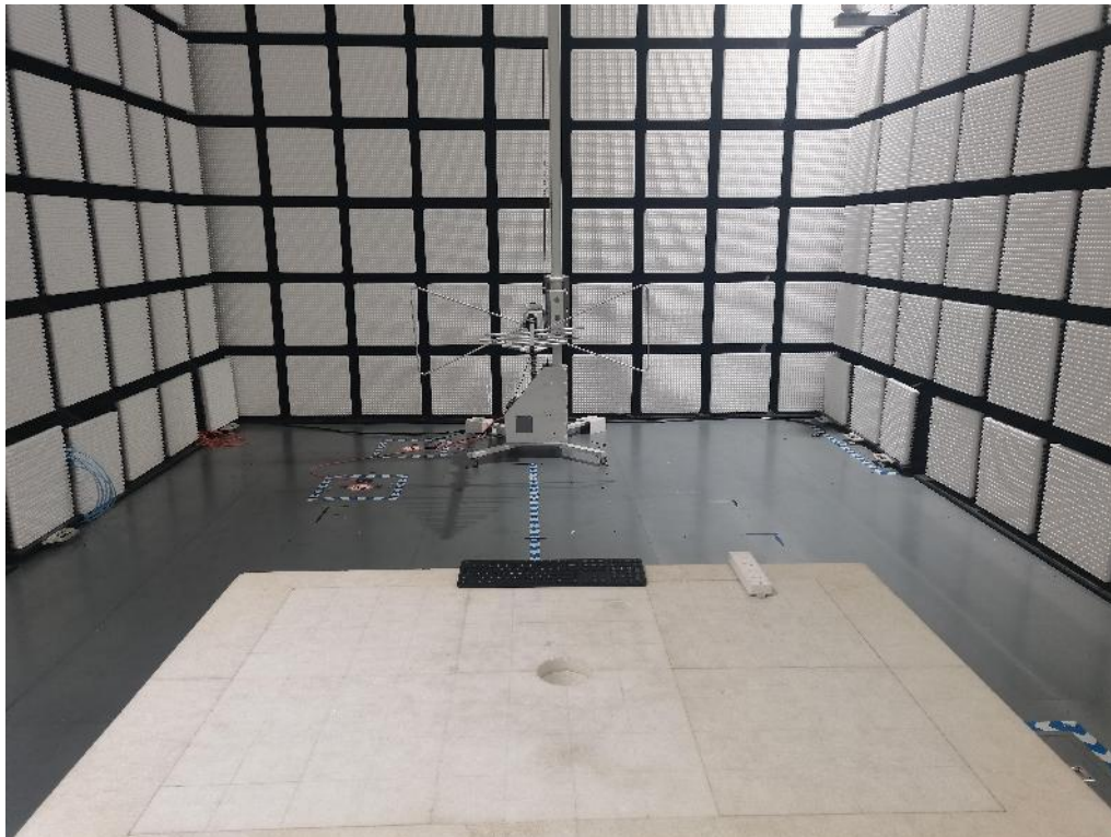
Fig. 2 Radiated emission setup photo(30MHz- 1GHz)
