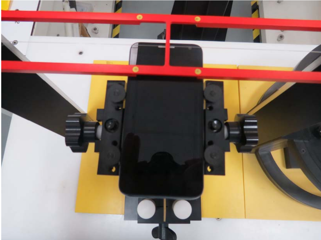
6036A HAC test setup photo RF Emission
