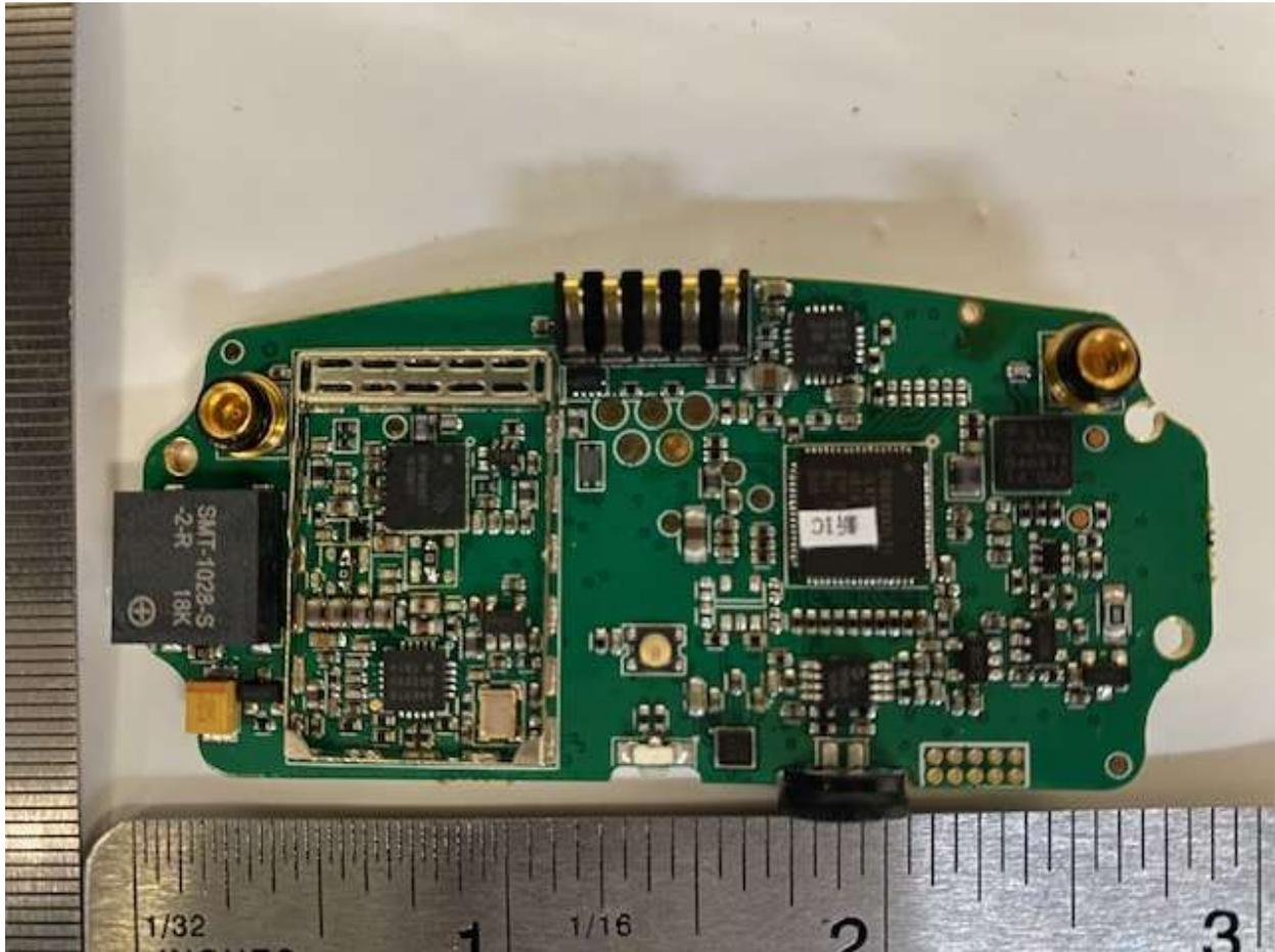
**Figure 9. PCB with Radio Circuit Shield Removed**
