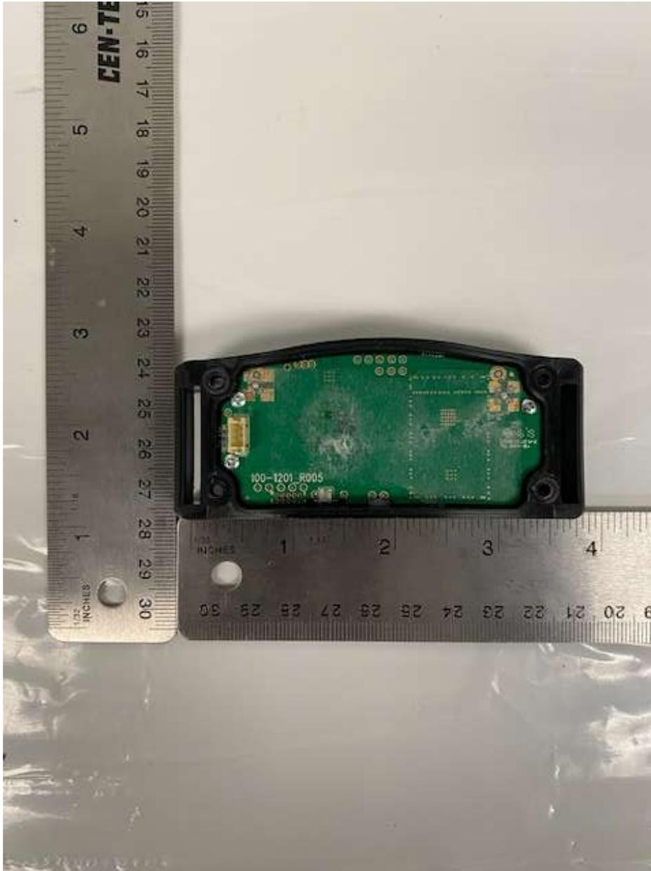
**Figure 5. PCB Mounted in EUT**
