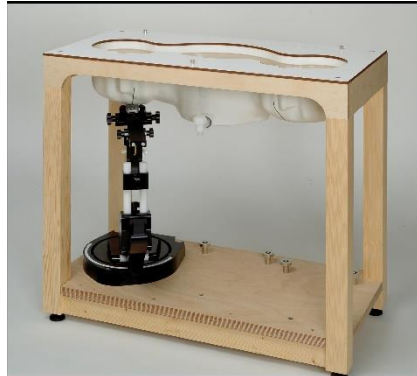
Picture C.10: SAM Twin Phantom
