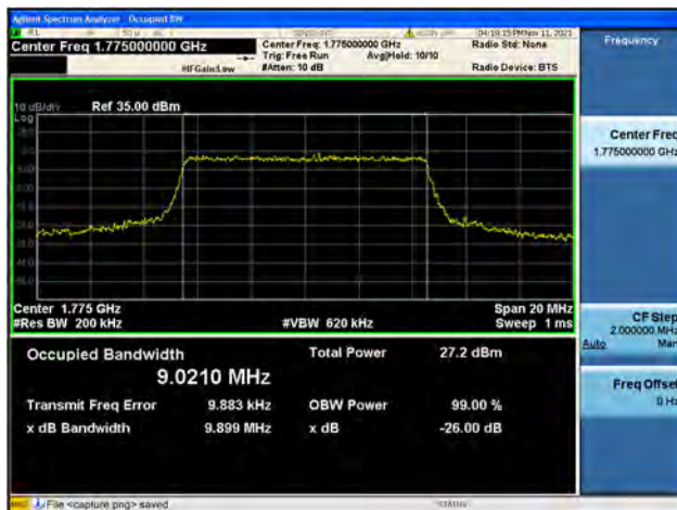
Band66 / 10MHz / High CH / QPSK
