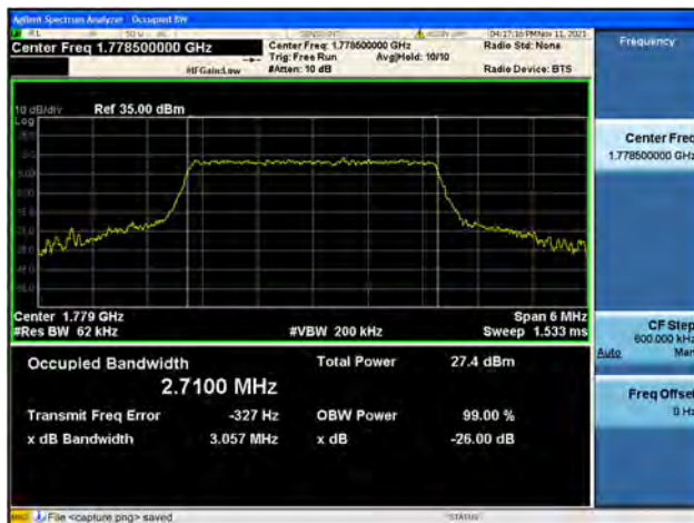
Band66 / 3MHz / High CH / QPSK
