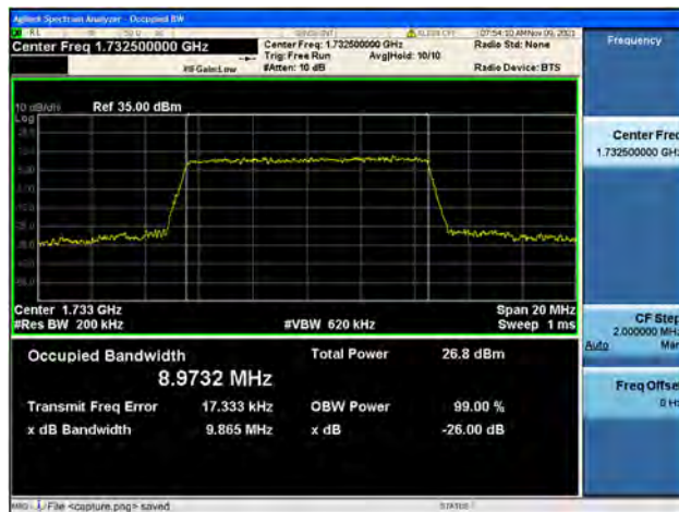
Band4 / 10MHz / High CH / QPSK
