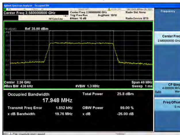
Band7 / 20MHz / High CH / QPSK
