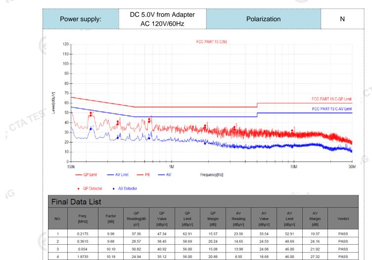
Note:1).QP Value ( $dB\mu V$ )= QP Reading ( $dB\mu V$ )+ Factor (dB)
