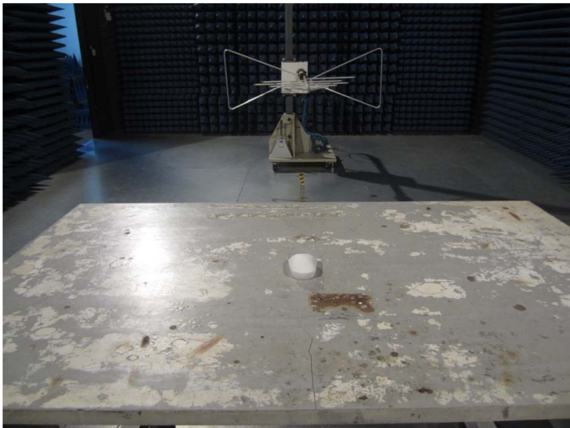
Setup photo for Radiated (below 1GHz):
