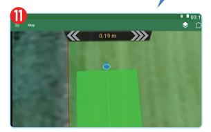
The changing value shows the offset distance, and the flash direction icon shows offset direction.
